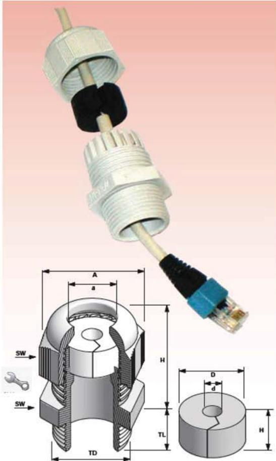
**Special design cable glands** with a split rubber seal. The cap and body holes are big enough to accept the RJ-45 connector. On the other hand the rubber inner diameter is small enough to provide a good seal, while a split still allows for cable insertion. During the application, the design supports assembly without having to disassemble the RJ-45 connector from the cable. This feature is also supported by the brass or EMC cable glands.
